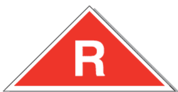
Building with Roof Truss Construction
