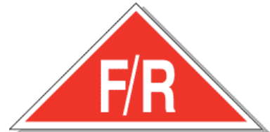
Building with Floor & Roof Truss Construction
