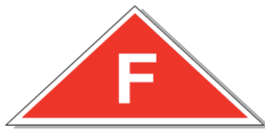
Building with Floor Truss Construction
